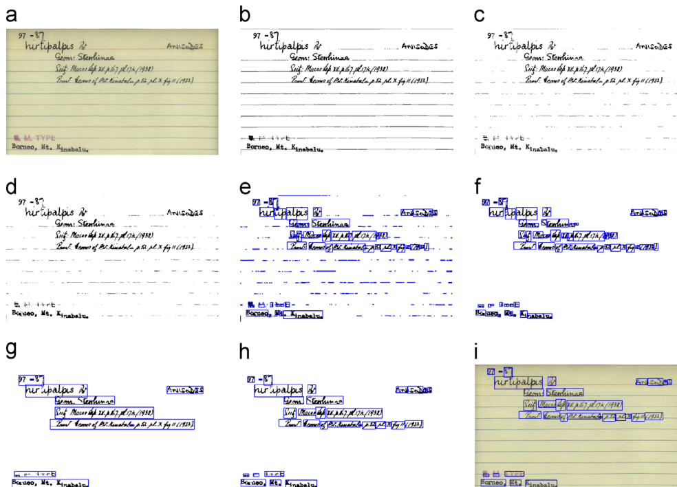
Fig. 5. (a) Original image, (b) binarized image, (c) graphical line removal, (d) morphological closing, (e) CCs before filtering, (f) CCs after filtering, (g) ARLSA output, (h) textual component detection, and (i) final results.
