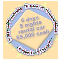
Fig. 2. A curved text line would be identified as a number of shorter straight lines.
