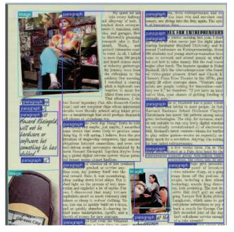
Figure 5. Example result of layout analysis by Tesseract 3.02.
