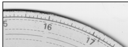
Figure 10. Shadow introduced by scanning
